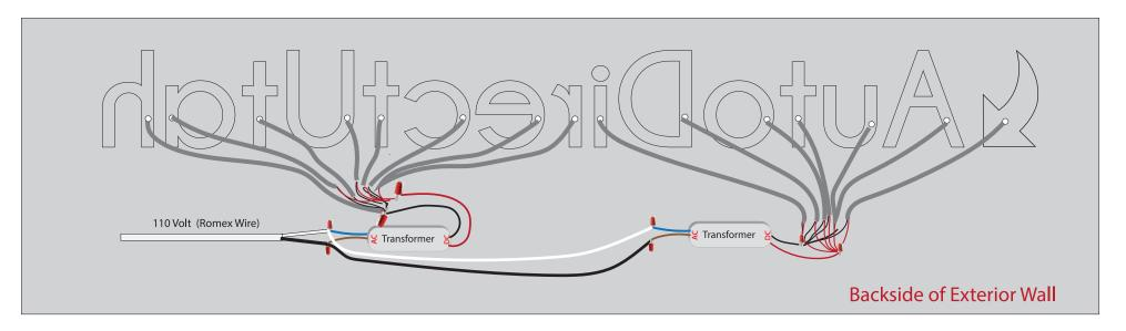
"always connect the wires from the sign to the transformer before connecting it to your power wire"
